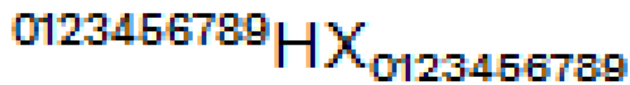
Figure 3.14: For comparison purposes, here the result with option --composites (and no ROUND_XY_TO_GRID ). The composite glyphs as a whole get hinted; consequently, the subscript glyphs get separate blue zones. At the displayed size of 16ppem the vertical positions of the subscript blue zones are rounded differently if compared to the superscript zones, thus the smaller glyph height.
