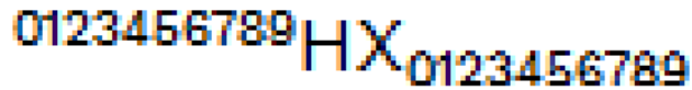
Figure 3.12: Here, the subscript glyphs are composites each having a single element that is shifted down. If option --composites is not used, subglyphs are hinted before they are glued together (possibly applying scaling and shifting). Because the ROUND_XY_TO_GRID flag isn't set, the vertical translation doesn't align the subglyph to the pixel grid, causing severe distortions.
