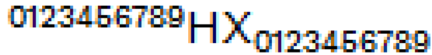
Figure 3.13: The same as before, but with ROUND_XY_TO_GRID set. Now the subscript glyphs look identical to the superscripts.
