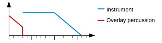
Since percussion instruments are often louder, this can help to create the illusion that both instruments have been played at the same time but the percussion instrument has drowned out the first couple of frames from the melodic instrument.
