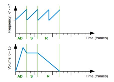
When a note starts, all frames of the Attack/Decay phase are played. Afterwards, the Sustain phase frames are played in a loop. When a pause note is encountered in the pattern, the Release phase frames are played once and the note ends in silence. If a new note is encountered instead of a pause, the new note simply cuts off the current instrument without sending it into Release phase.
