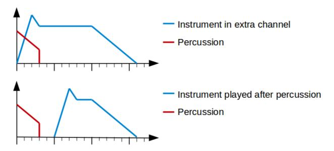
The top picture shows the ideal situation, where the melodic and percussion instruments are played simultaneously in different channels. The bottom picture shows what happens if the composer plays them one after the other in the same channel. In this example with a song tempo of 5, you have a gap of two ticks after the percussion has finished before the next note is played.
