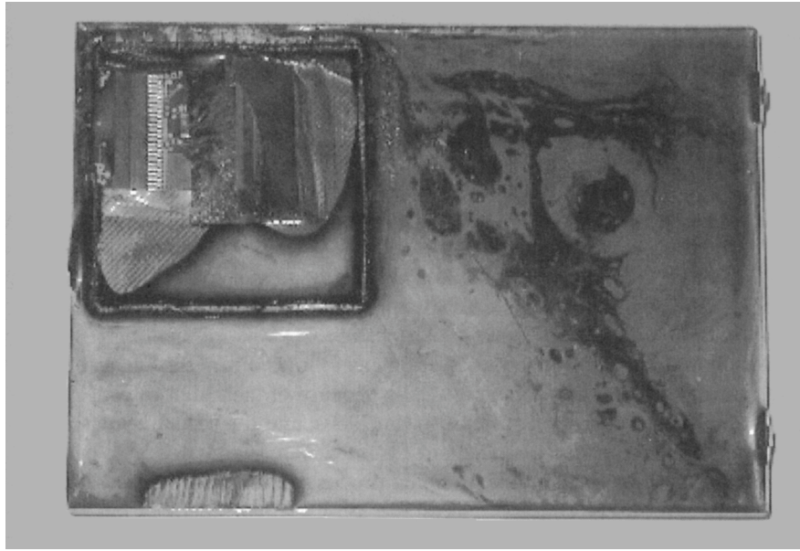
Figure 14.2 The 4758 partially opened, showing (from top left downward) the circuitry, aluminium electromagnetic shielding, tamper-sensing mesh and potting material (courtesy of Frank Stajano).
